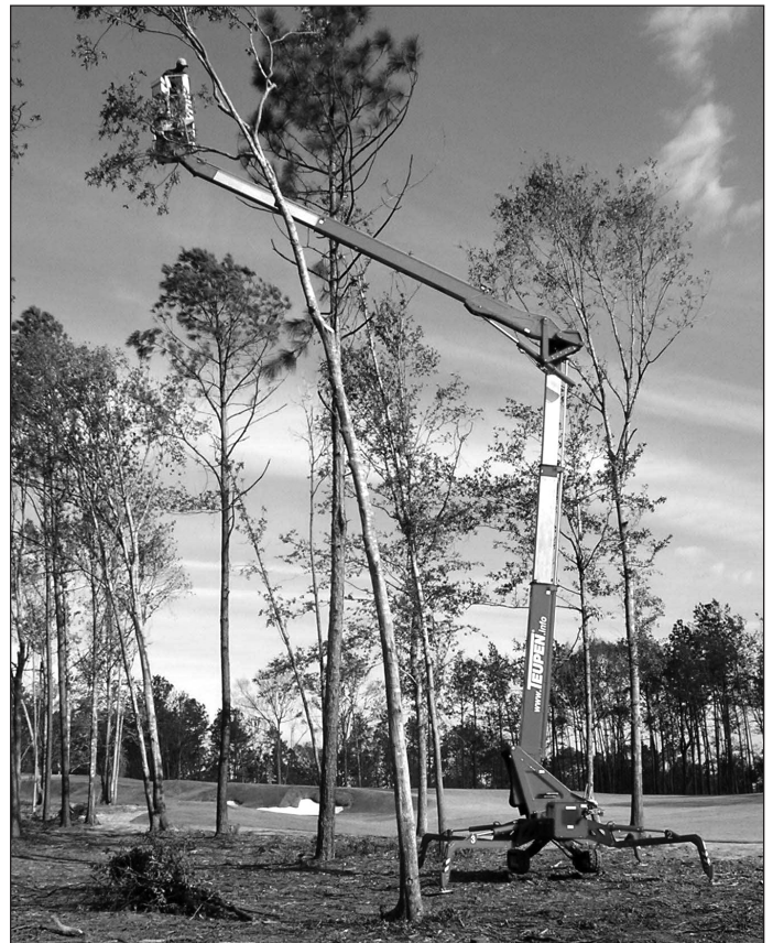
Today, mini aerial lifts can maneuver in parks and yards while safely raising tree pruners as much as 150 feet or more.
