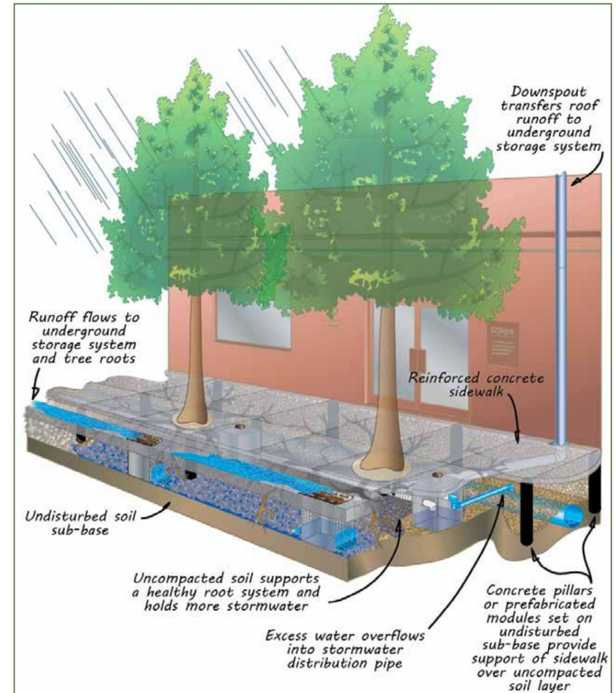
**Above:** Suspended sidewalks use pillars or structured cell systems to support reinforced concrete, increasing the volume of uncompacted soil in subsurface planting areas and enhancing both root growth and stormwater storage.
