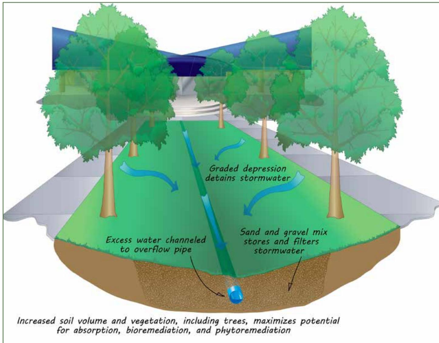
**Above:** Bioswales are landscaped drainage areas with gently sloped sides designed to provide temporary storage while runoff infiltrates the soil. They reduce off-site runoff and trap pollutants and silt.
