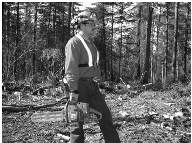
Carry the chain saw at your side with the bar pointing back and with the engine off or the chain brake set.
